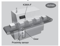
Monitoring line speed for a reflow furnace
